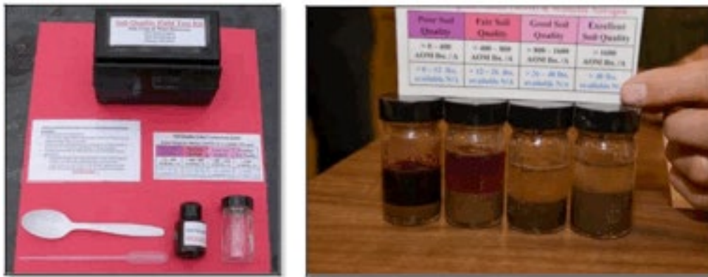
Fig. 1 Field kit for in-situ active C test ( https://go.osu.edu/SoilTestKit )
