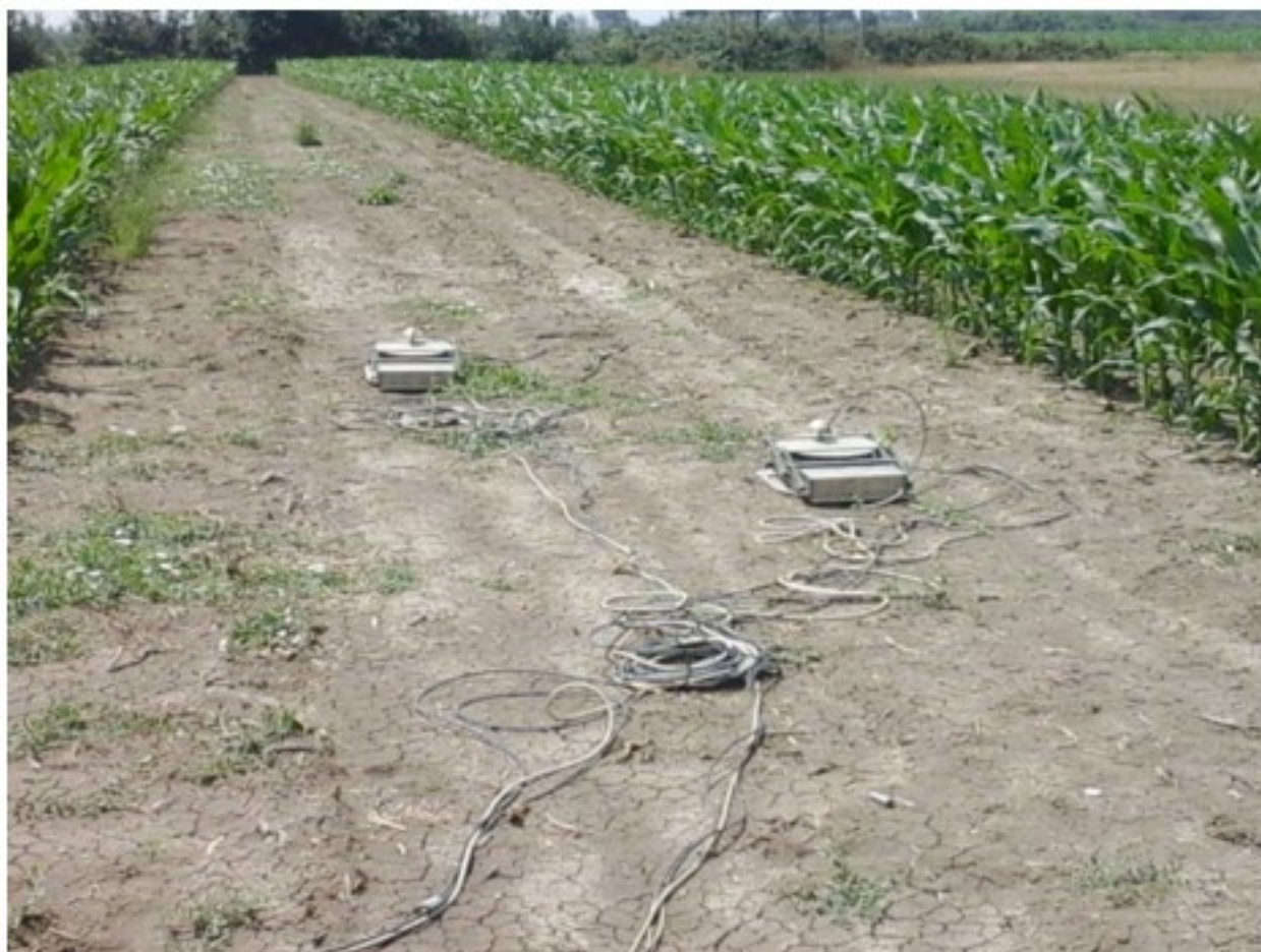
Figure 1. GHG field sampling system
