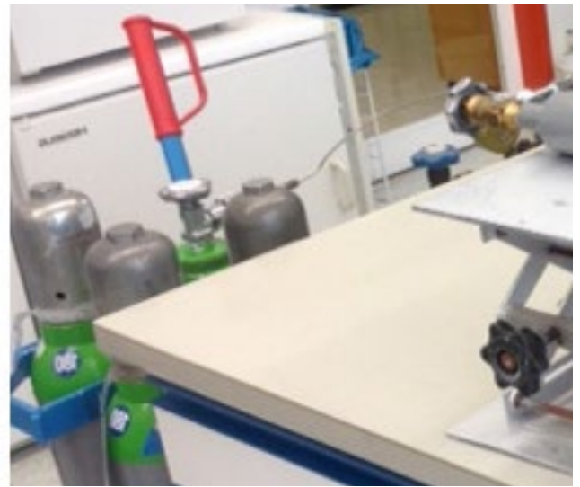
Fig. 1: Gas mixing line (left) linked to a vacuum pump, pressure gauge, CO 2 and synthetic air gas tanks for mixing of gases into desired containers, such as this 1L gas cylinder, to make standard reference gases for laser isotope analyzers; 13C - CO 2 laser isotope analyzer (right) for measuring emissions of CO 2 from soils.
