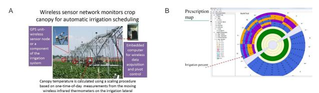
**Figure 2.** (A) A variable rate irrigation (VRI) center pivot system combined with a wireless network of crop canopy temperature sensors (thermal infrared) and soil water sensors used by the ISSCADA system to automatically determine full and deficit irrigation levels and control the VRI system at the USDA, ARS Conservation & Production Research Laboratory, Bushland, Texas. (B) Example of a prescription map produced by the ARSmartPivot software.
