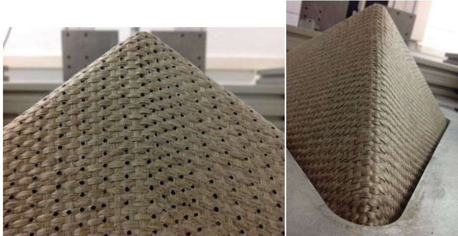
FIGURE 8 : Un-balanced plain weave fabric without tow buckles
