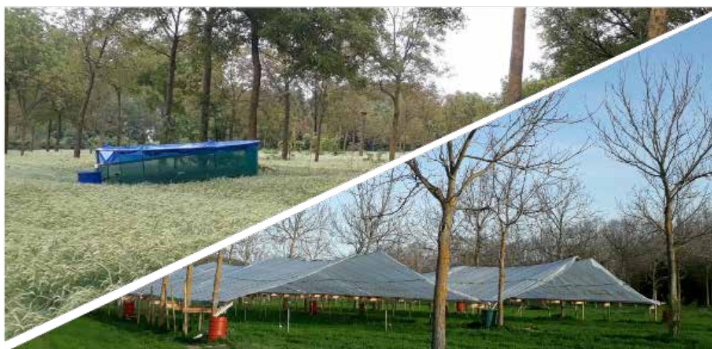
Rainout shelters at the Restinclières Farm Estate: on the left, a prototype that aims at excluding rainfall at the crop scale solely ; on the right, another prototype that aims at excluding rainfall for both the crop and the trees.
