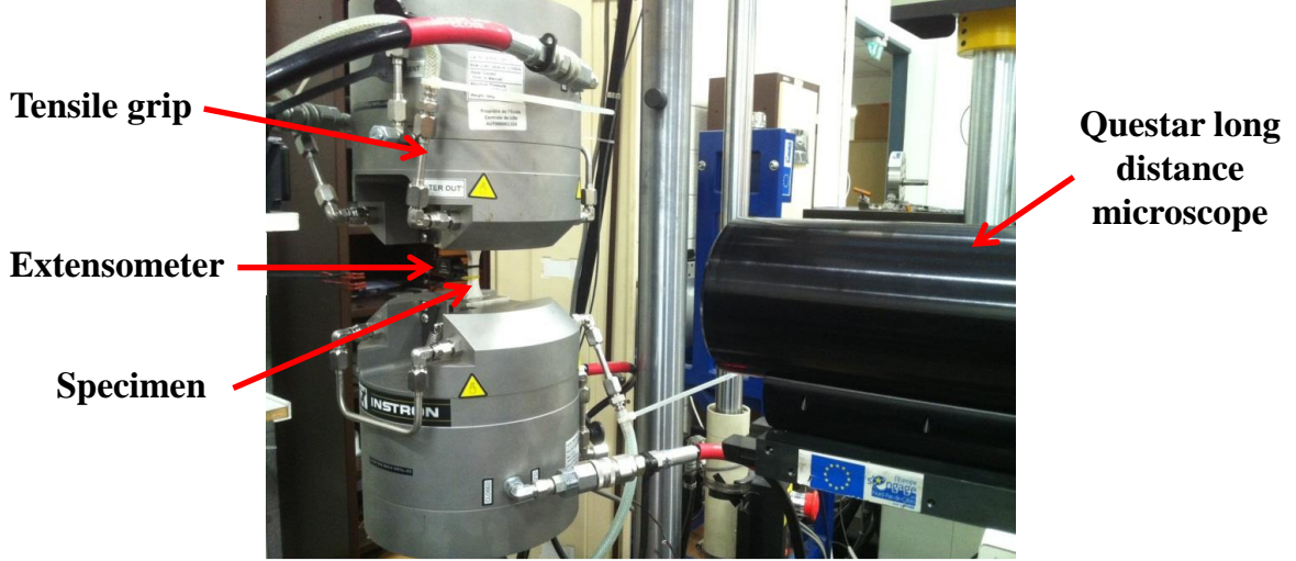
Figure 2: Experimental set-up with Questar microscope.
