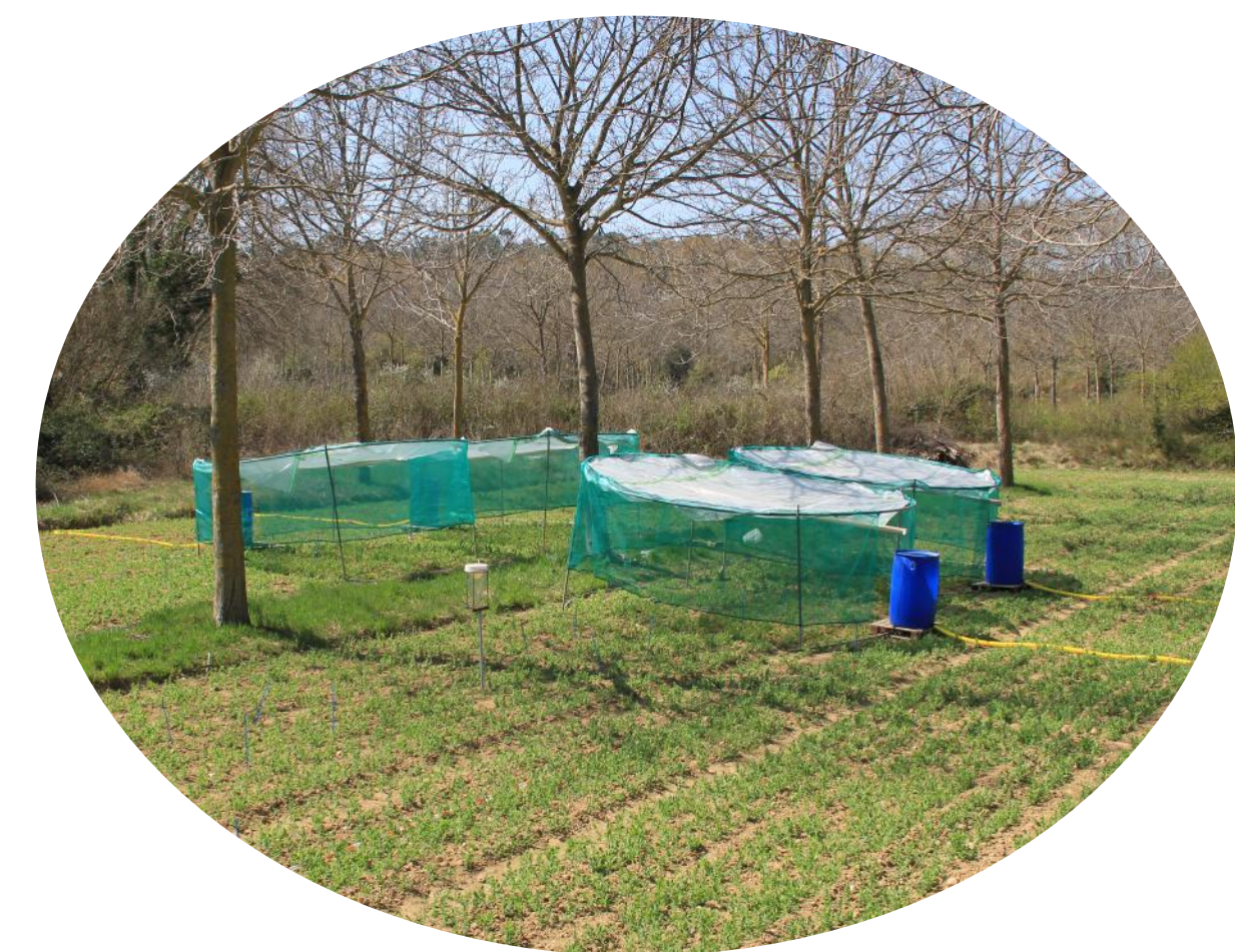
Tubular structure with removable roof. 4 rainout shelters around a tree (~4x15m 2 ).
