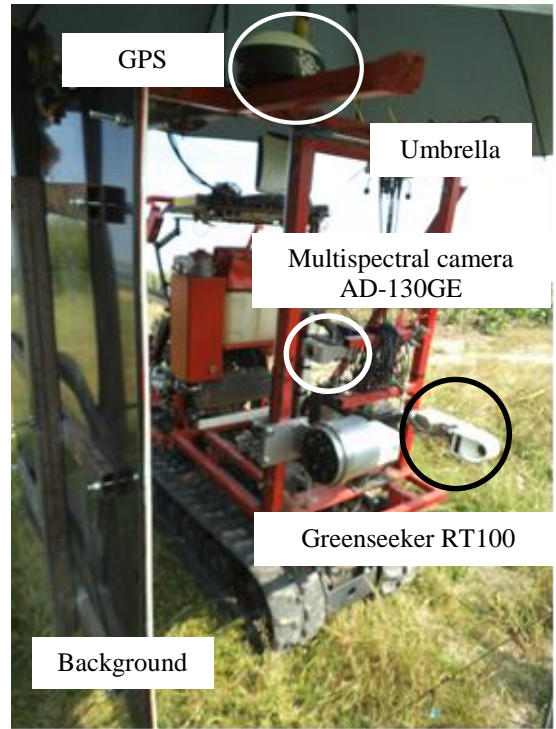
Fig. 2. The multispectral camera, Greenseeker and the GPS embedded on the track laying tractor
