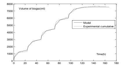
Figure 1.Comparison of the experimental and modeled biogas production for carrot at an OLR of 0.5g VS/l/d.
