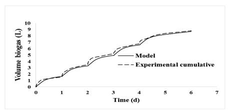
Figure 3. Modelling with modified ADM1 model for carrot at an OLR of 0.5 g VS/L/d.
