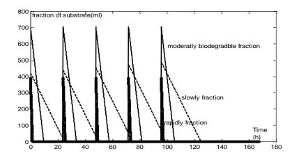
**Figure 2.** Evolution during one week of the three biodegradable fractions for carrot at an OLR of 0.5 g VS/L/d.
