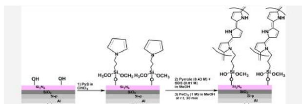
**Scheme 1.** Schematic representation of: (a) activated Si<sub>3</sub>N<sub>4</sub>, (b) Si<sub>3</sub>N<sub>4</sub>-SPy, and (c) the development of Si<sub>3</sub>N<sub>4</sub>-P(SP<sub>3</sub>-Py) compound materials.
