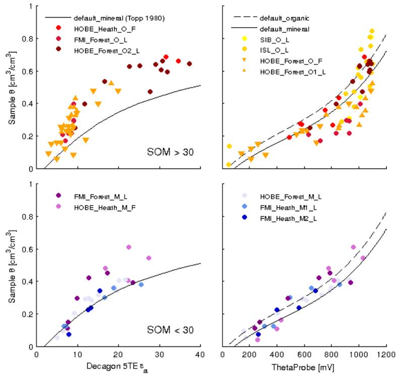
Figure 2: 5TE apparent dielectric constant  $\epsilon_a$  (left) and ThetaProbe output [mV] (right column) against volumetric water content  $\Theta$  (gravimetric samples) for organic (top) and mineral horizons (bottom row) with color codes from highest to lowest SOM content (yellow – dark red and purple - dark blue, respectively). For SOM% see Table 1.
