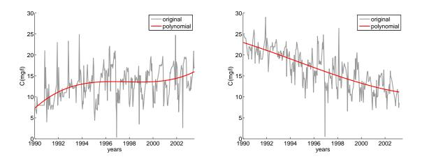
Figure 1: Measured nitrogen concentration  $C_1^N(t)$  and  $C_2^N(t)$  in two similar sources  $S_1$  and  $S_2$  along with a 3<sup>rd</sup> order polynomial approximation  $M_1^N(t)$  and  $M_2^N(t)$
