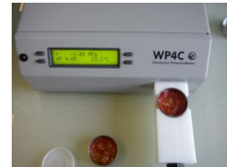
Fig.3: WP4C device with cut slices of mature fruits
