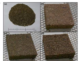
Fig. 3. Photographs of the cake (a) and of the three fiberboards with 25% binder content (b, board S4; c, board C4; d, board G4).
