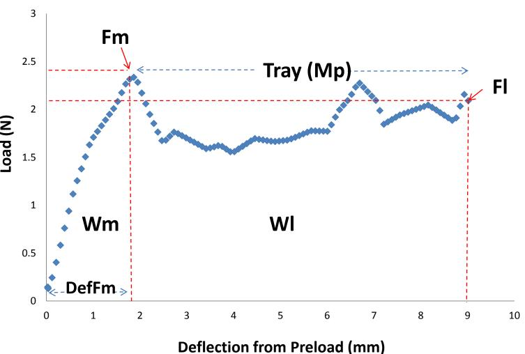
Localization of the puncture tests and parameters obtained according the force / displacement curve. Fm (N): maximum load, DefFm(mm): deflection at maximum load, Wm(J): work to maximum load, Fl(N): load at limit, Wl(J): work to limit, Mp (N): load average for the tray.
