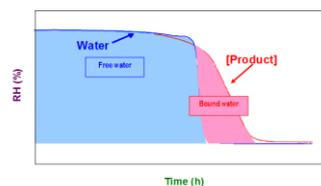
Fig. 1 – Kinetics of drying by desorption
