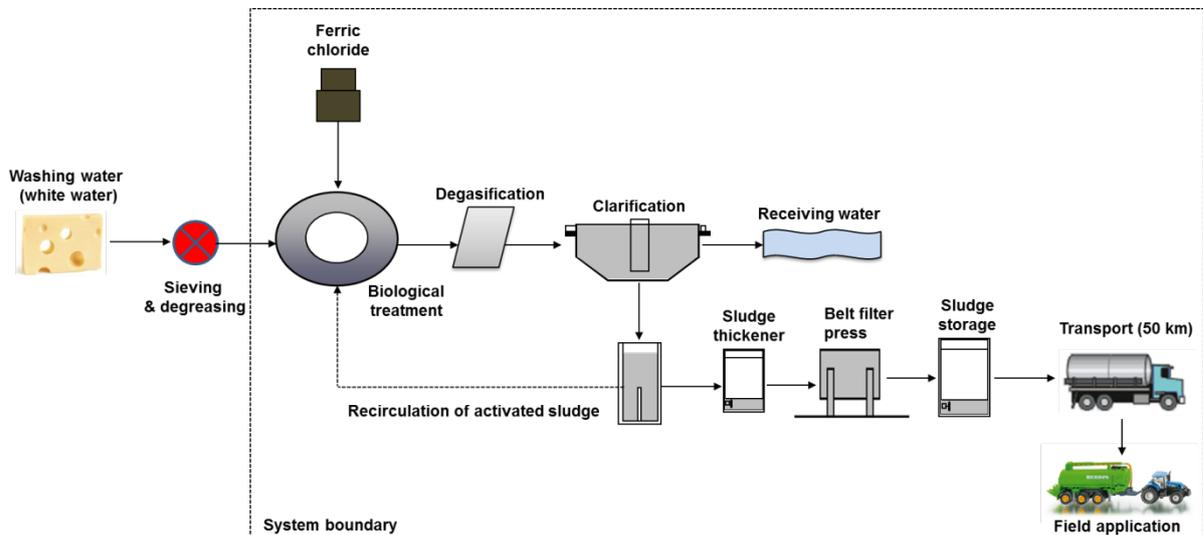
**Figure 1.** Schematic of the treatment process for washing waters from cheese production.
