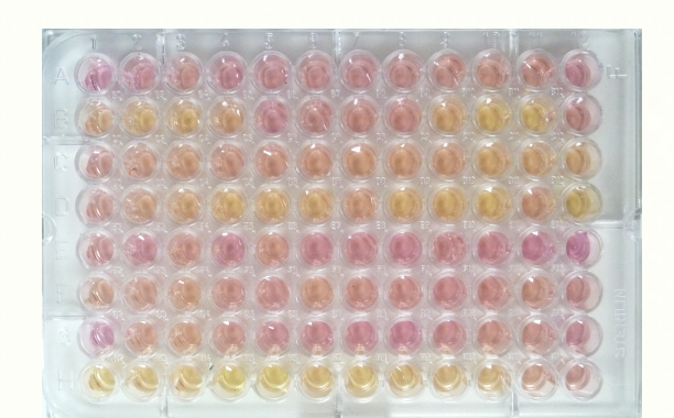
Figure 1 : Photograph of the Cresol Red gel detector CO 2 -trap microplate after incubation with soil and substrate
