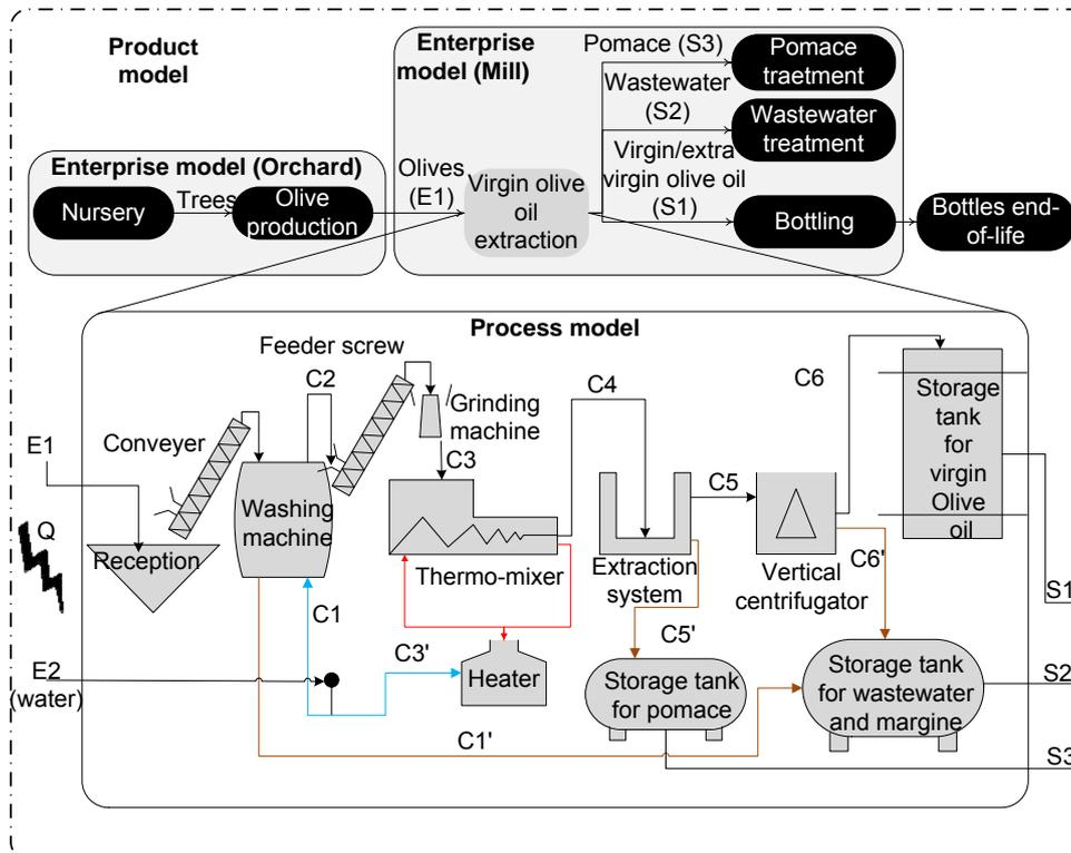
Figure 3: Olive oil production system
