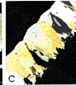
Old hen egg Breaking strength: 4 N Thickness: 360 \mu\text{m}
