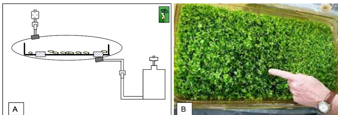
**Figure 3.** Horizontal disposable Temporary Immersion Bioreactor (“Box-in-Bag”): a) diagram, b) view of a culture of pregerminated Robusta somatic embryos after 2 months.
