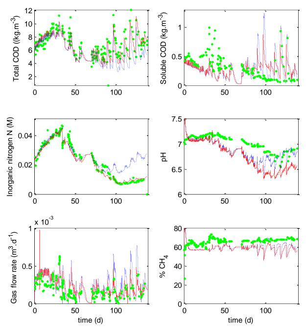
**Figure 2.** Comparison between the original ADM1 (blue dashed lines), the modified ADM1 (red lines) and experimental data (green dots) of *Chlorella vulgaris* digestion.
