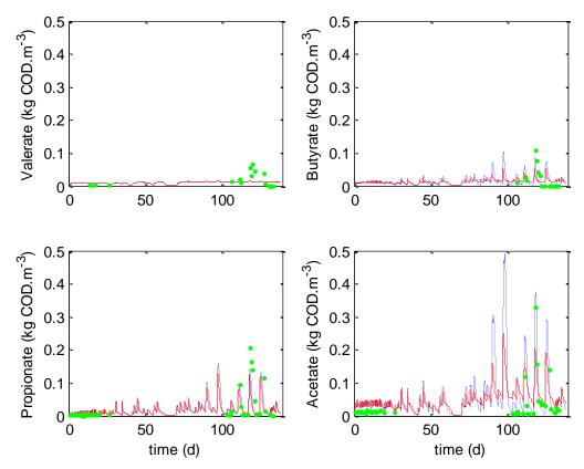
**Figure 3.** VFA concentrations: comparison between the original ADM1 (blue dashed lines), the modified ADM1 (red lines) and experimental data (green dots) of *Chlorella vulgaris* digestion.
