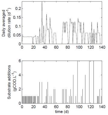
Figure 1. Operating conditions for the anaerobic digestion of the freshwater microalgae *Chlorella vulgaris*.
