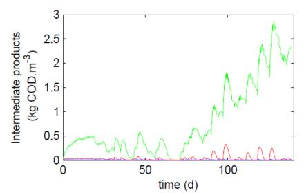
**Figure 4.** Model prediction of carbohydrate (blue line), protein (green line) and lipid (red line) concentrations during *Chlorella vulgaris* digestion. The high dilution rate at the end of the experiment leads to an accumulation of proteins.
