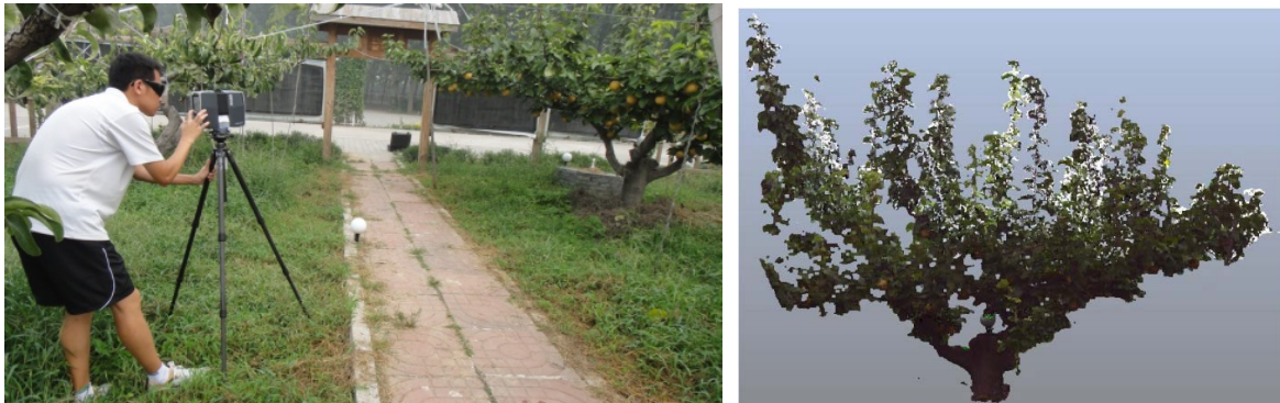
Fig. 1. Scanning pear tree by using FARO Laser Scanner Focus3D(left); the measured colored point cloud(right).
