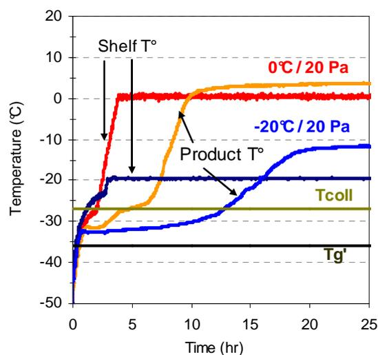
**Figure 4.** Shelf and product temperature profiles obtained during the sublimation step of the two freeze-drying cycles performed to validate the “biological model”. The values of the collapse temperature ( $T_{coll}$ ) and the glass transition temperature of the maximally freeze-concentrated phase ( $T_g'$ ) of the protected bacteria suspension are also reported.
