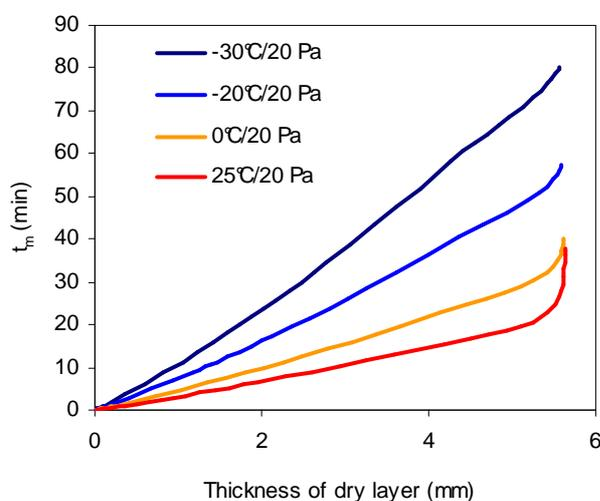
**Figure 3.** Simulation results of the evolution of the acidification activity ( $t_m$ ) of lactic acid bacteria during the freeze-drying process for various operating conditions applied during the sublimation phase. The initial  $t_m$  value was arbitrarily fixed at zero at the beginning of the process.
