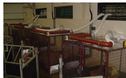
Figure 1 Chambers to measure methane emission from small ruminant
