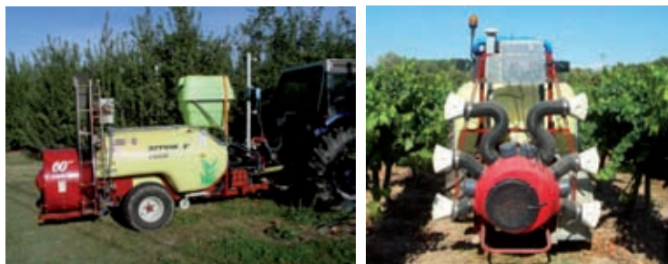
Fig. 2. Variable rate prototype sprayer for orchards (left) and for vineyards (right).
