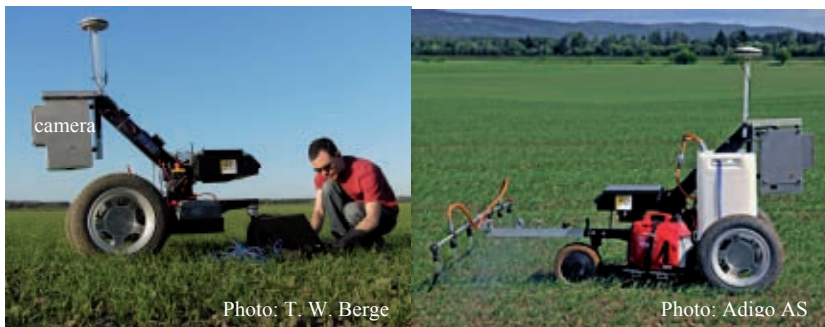
Fig. 1. GPS-guided robot used for R&D in machine-vision based site-specific weed management (SSWM) in small grain cereals. Left: Sampling of imagery for machine vision developments and map-based SSWM. Right: Robot conducting real-time SSWM with a 3-m wide spray boom (forward direction is to the right).
