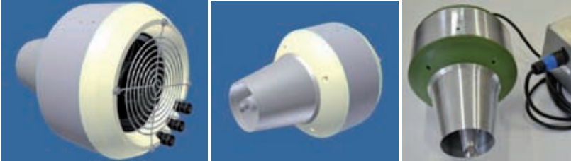
Fig. 1. Close range precision spraying end effector (SEF). Left: back view of the model, middle: front view of the model and right: manufactured SEF with control box.
