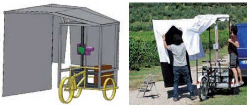
Fig. 1. Instrumented field trolley hosting the acquisition system. Canopy imaging is done inside a tunnel structure providing background regularization and diffuse illumination of the measured area
