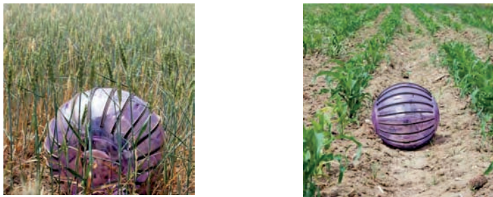
Figure 2: ROSPHERE measuring enviromental variables. a) In winter cereals b) corn crops
