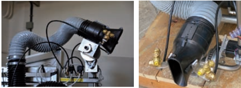
Fig. 6 – tilt diffusor ( left ) with double nozzles ( right ).
