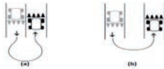
Fig. 1. Manoeuvres in the headland turns (a) loop turn, (b) double round corner.
