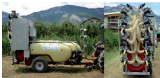
Fig. 1. ISAFRUIT CASA sprayer prototype equipped with CIS and EDAS systems.
