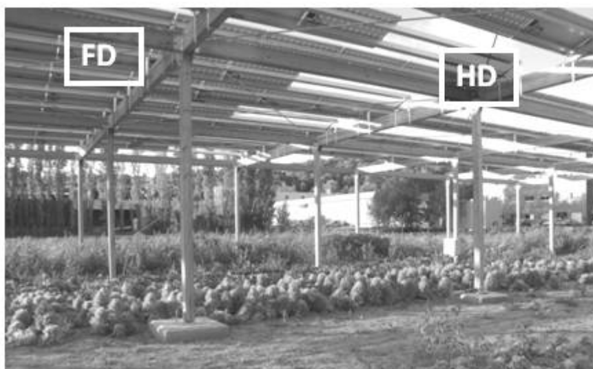
Figure 1: Experimental AVA in Montpellier (France). FD and HD subsystems are visible respectively on the left and the right parts of the picture. Photographie C. Dupraz, INRA.
