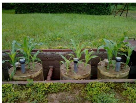
Figure 2. Sampling of gas and surface CO 2 flux from soil columns during the vegetation season from 13 th April till 1 st September (0 = control; NPK = NPK treatment; M = presence of maize plant; FYM= farmyard manure).
