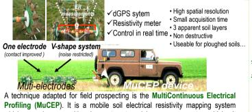
**Profiling (MuCEP)**. It is a mobile soil electrical resistivity mapping system which comprises a multi-probe system towed by a cross-country vehicle. It cover a large area in few time and measure field resistivity at high resolution. (ARP patented, Geocarta society, Paris, France)
