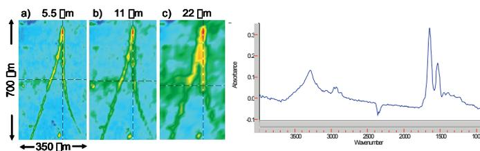
Rat brain cross-section images were collected on an Agilent Cary 670 FTIR spectrometer and Cary 620 infrared microscope equipped with a 64x64 MCT FPA. All images were acquired at 8  $\text{cm}^{-1}$  spectral resolution with
