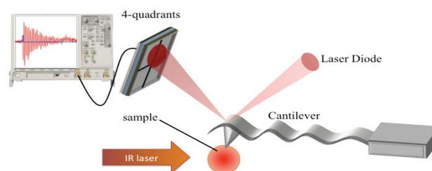
**figure n°1 : scheme of the AFMIR technique**
