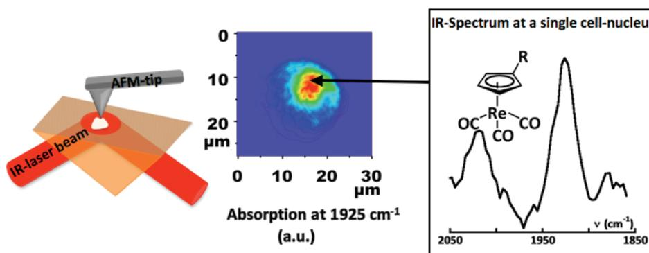
On the left, prism illuminated by the IR-beam with deposited cell and AFM-tip in contact. In the middle, chemical mapping at one CO-vibration band
