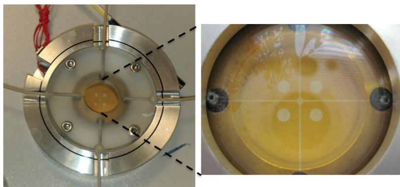
Figure 1: Example of a 3D microfluidic device made in XARP resist on CaF<sub>2</sub> allocated within the chip holder, manufactured in order to allow i- the connections with syringe pumps through microcapillaries for supply/waste of cells and chemical ii- the chip thermalization through an heater, made by a resistor embedded in an aluminium cylinder.
