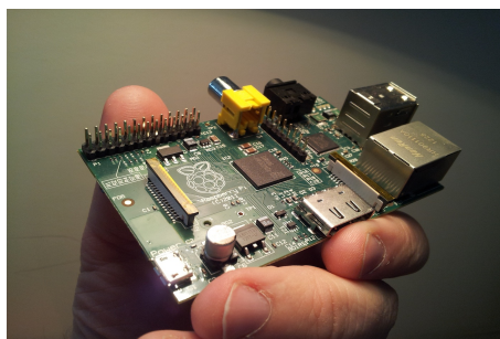
Figure 1. The Raspberry Pi is a low-cost (35€) credit-card sized computer.
