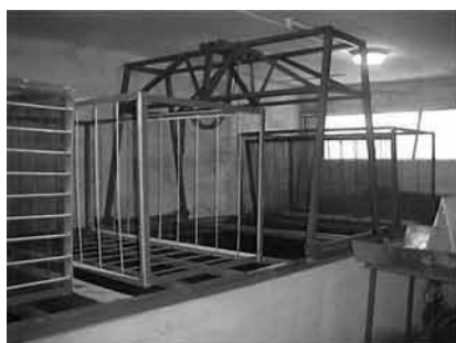
Tanks, cages and cranes used in the soaking and pasteurization process
