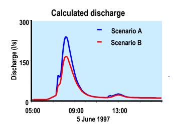
Figure 4. Example of the impact of scenarios of land use change A and B on the simulated hydrograph on the Roujan catchment.
