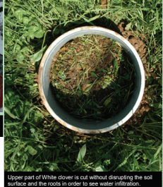
Simplified Beerkan test. Cumulative time for water infiltration is measured through a cylinder (30cm diameter).
