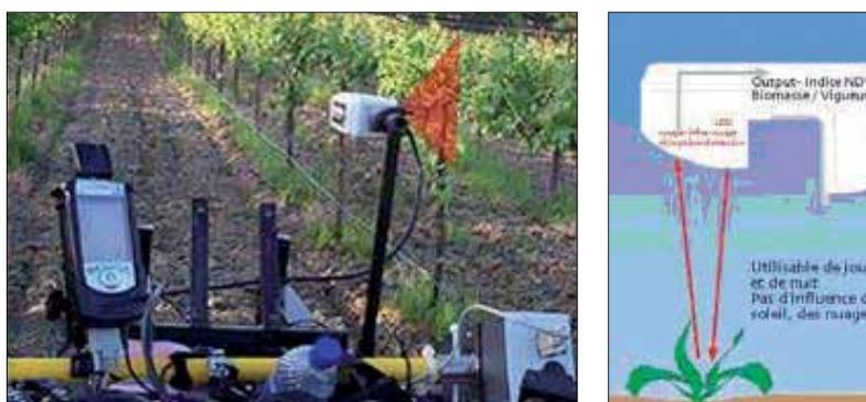
Figure 8 : Capteur Greenseeker, installation (source [http:// www. ntechindustries.com](http://www.ntechindustries.com))
