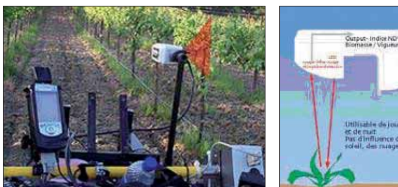
Figure 8 : Capteur Greenseeker, installation (source http:// www. ntechindustries.com )
