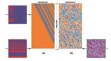
Numerical calculations of our cellular automaton model. The direction of every individual is fixed to the left. (a) With no scooping; (b) With scooping. The temporal variation of the waving state is plotted for the individuals of the 50 th row in the 2-dimensional lattice space.
