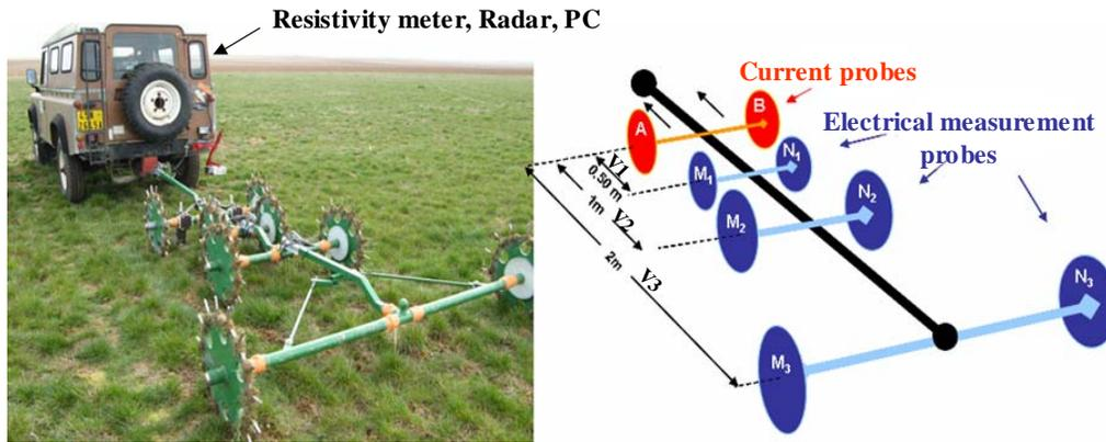
**Figure 2:** The Multi-Continuous Electrical Profiling device (MUCEP).
