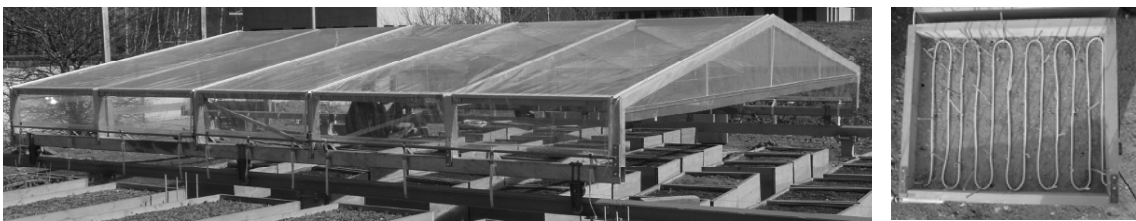
Figures 1 & 2: Experimental set-up. Automatic rainshelters cover seed/seedling beds during rainfall (left). Heating cables increase actual soil temperatures by 0 K, 2.5 K and 5 K, respectively (right).
