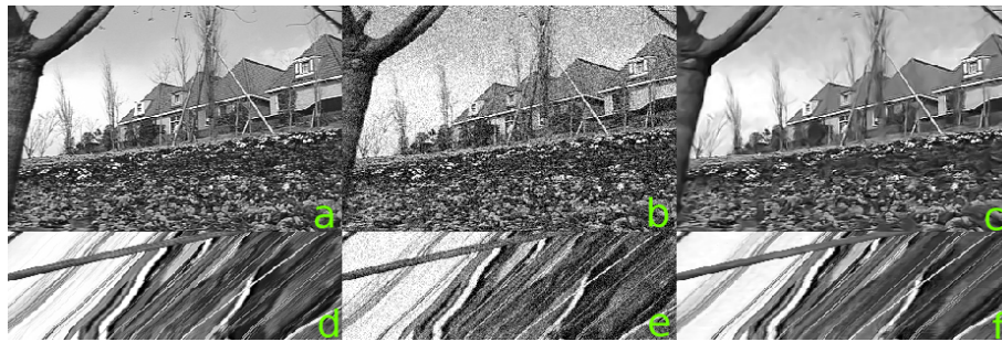
Fig. 5. Sequence “Garden”. (a) original sequence, (b) noisy sequence with a additive Gaussian white noise of standard deviation \tau = 30 ( PSNR = 18.58dB ) and (c) denoised sequence, PSNR = 23.59dB . (d), (e) and (f) represent corresponding XT slices in space-time domain. The camera motion appear as lines in the XT slices.
