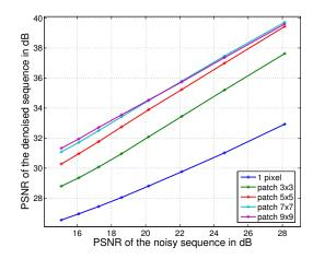
**Fig. 3.** Denoising performance for several noise levels and for several patch sizes. The PSNR is used to measure the overall performance of the filtering and the test sequence is Akyio ( $176 \times 144 \times 300$ ). This sequence mainly exhibits low motion. Experiments show that the introduction of patches improve the PSNR of at least 2dB. We can also remark that the results for patch  $7 \times 7$  and  $9 \times 9$  are similar.
