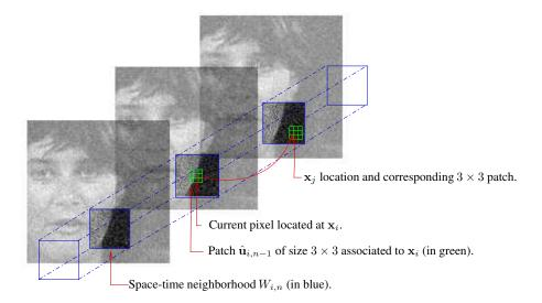
Fig. 1. Exemplar-based space-time approach. To each point of the image sequence is associated an estimated space-time neighborhood  $W_{i,n}$ . To each point  $\mathbf{x}_j$  of this neighborhood is associated a  $3 \times 3$  patch. The weights  $\omega_{ij}$  are defined as a function of the distance between the patch centered in point  $\mathbf{x}_i$  and patches centered in point  $\mathbf{x}_j \in W_{i,n}$ .
