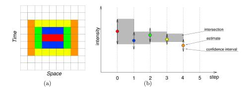
**Fig. 2.** (a) Spatio-temporal neighborhood: colors correspond to iterations plotted in (b); (b) confidence intervals: circles represent estimates  $\hat{u}_{i,n}$  obtained at each iteration n. The gray rectangles represent the intersection between the current confidence interval and the previous one. As long as the estimate belongs to this intersection, the estimation process is updated.
