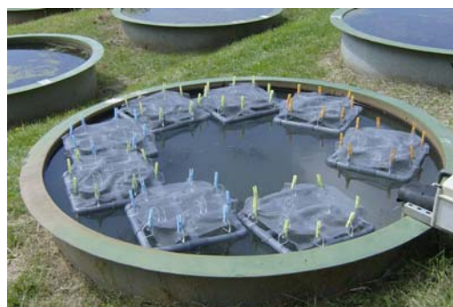
Figure 1: Experimental design. For this study, we capitalized on a large-scale experimental evolution set-up at the University of Liverpool. We installed 36 enclosures (7-liter) in a heated mesocosm.
