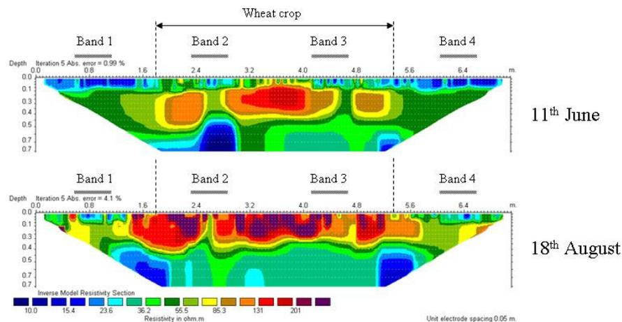
**Figure 10.** 2D ERT measured along the line III (a) the 10<sup>th</sup> of June 2009 and (b) the 18<sup>th</sup> of August 2009. Grey lines (Band 1, 2, 3 and 4) show the location of compacted zones.
