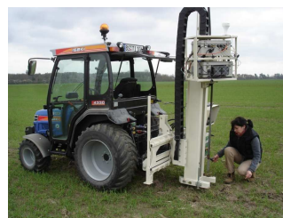
Figure 2. The Veris-Probe with the foot as a robust column that connects the hydraulic arrangement with the NIR-drilling rod and window, the spectrometer and auxiliary case, the GPS.
