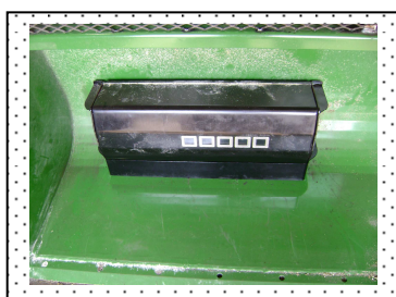
Figure 1. Scanner Unit inside the bucket of the Front
