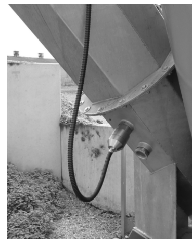
Figure 3. TENferm measuring head installed in a silage auger (top), sampling plug (below)
