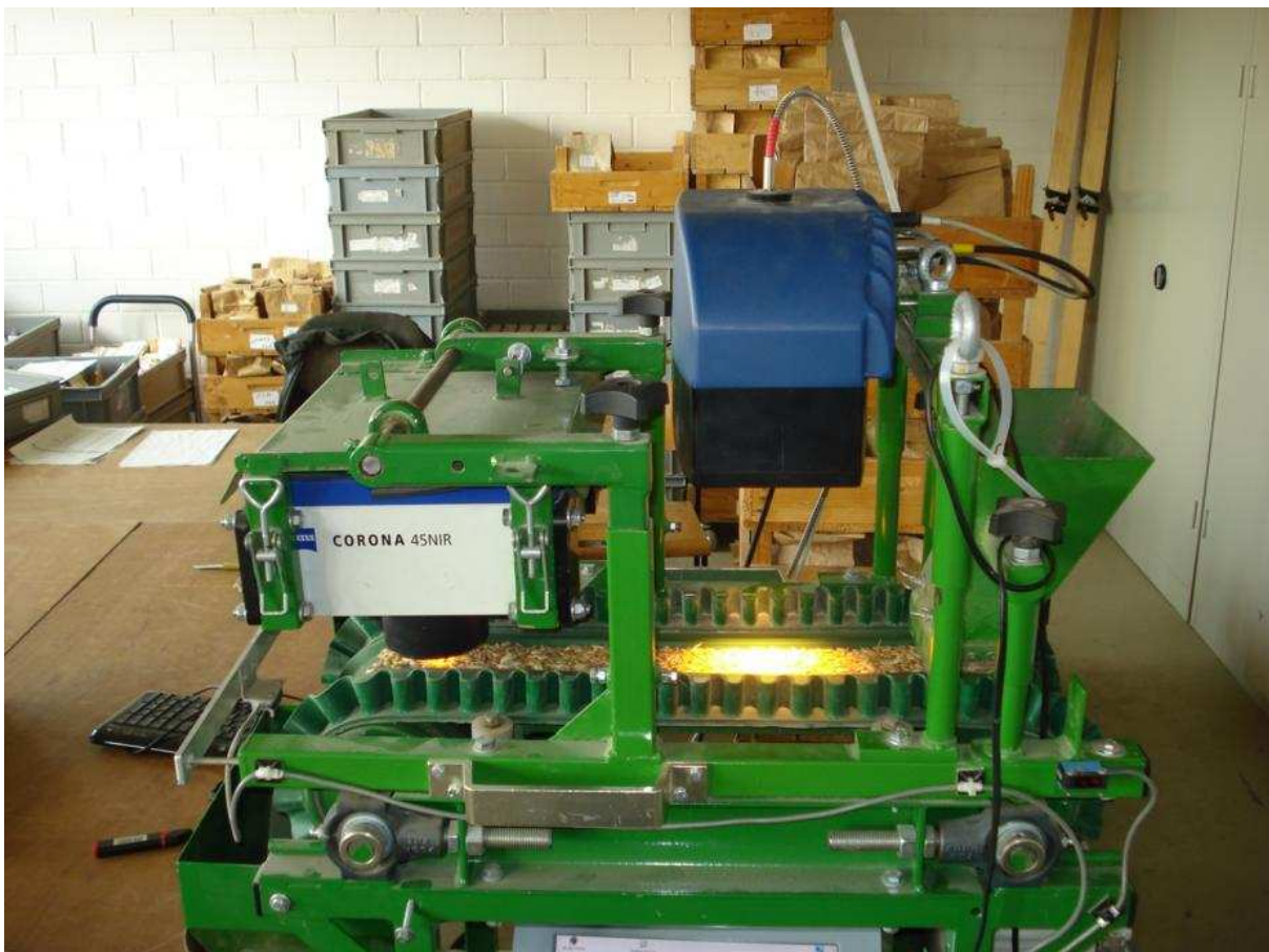
Figure 1. Combined at-line system with Zeiss Corona and Polytec NIR spectrometer.
