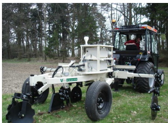
Figure 1. The Veris-shank with optical unit, the subsoiler chisel, six blade coulters for measuring electric conductivity, the spectrometer and auxiliary case, two closing discs, the GPS.
