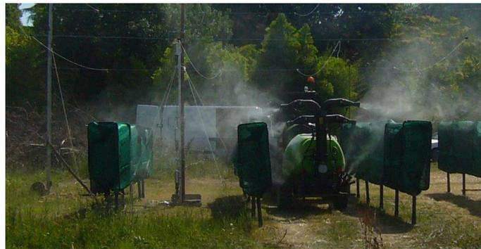
Fig. 7: Illustration of the upward direction of the lower jet of the sprayer.
