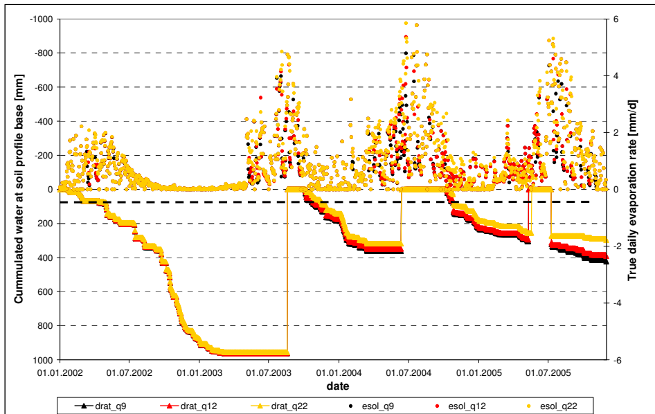
Figure 2: Effect of using different approaches to estimate evaporation: regarding cumulated water at soil profile base and true daily evaporation rate.
