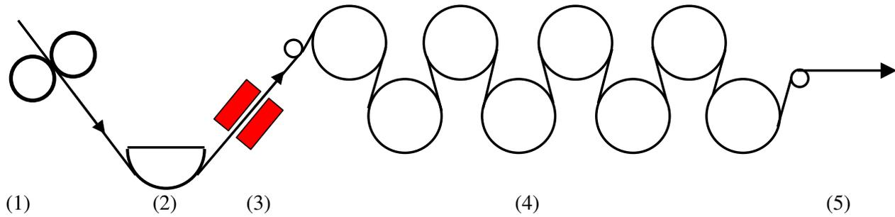
Figure 2 - Layout description of the example used in this section: 1) Coater, 2) Convective Free Draw (including a non-contact deviator), 3) Infrared section: 1 m, face to face, 250 kW/m<sup>2</sup> by face, 4) Conductive section: 8 steam heated cylinders of 1.5 m diameter and 5) Convective section: Free Draw of 4 m.
