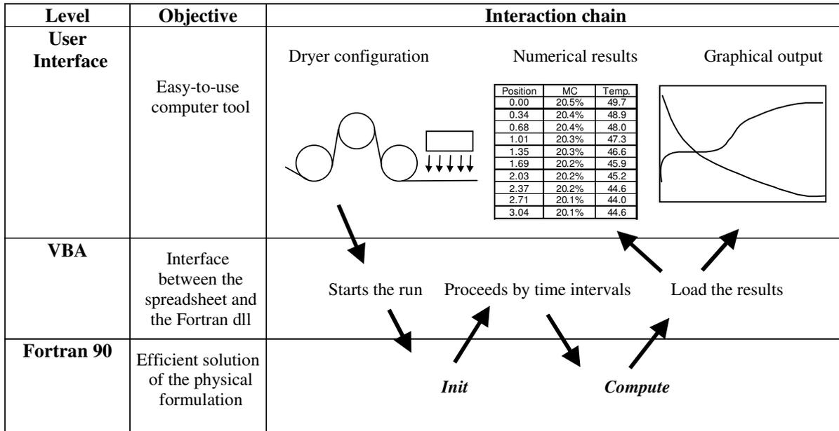
Fig. 1 – The structure of the new simulation tool.
