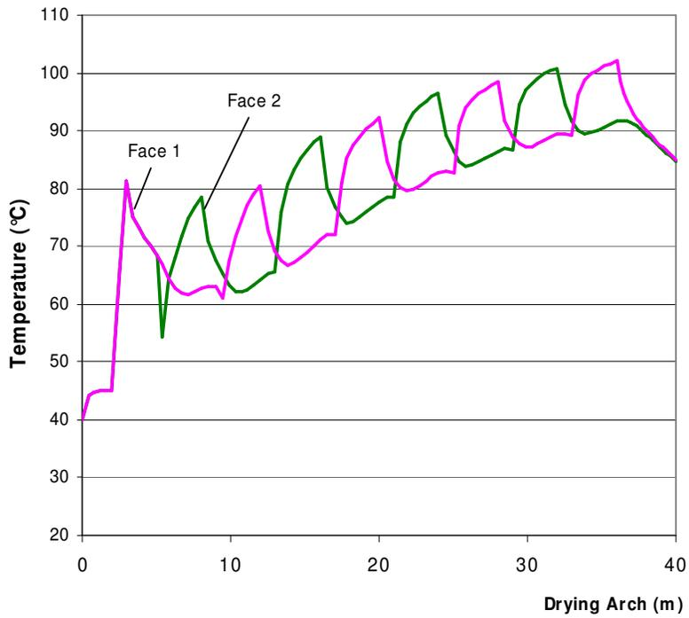
Figure 4 – The evolution of the surface temperature of each face along the dryer.
