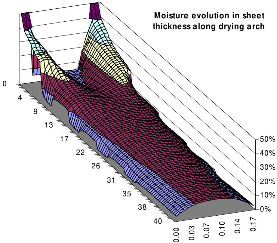
Figure 5 – The evolution of the moisture content profile in the three layer support the dryer.
