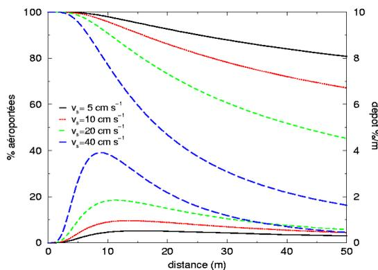
Figure 2. Influence of the sedimentation velocity on the deposition (bottom curves) and the remaining fraction of the initial horizontal flux (top curves). In this simulation the source height is 3 m,  $u_* = 0.3 \text{ m s}^{-1}$  and  $z_0 = 0.05 \text{ m}$ .
